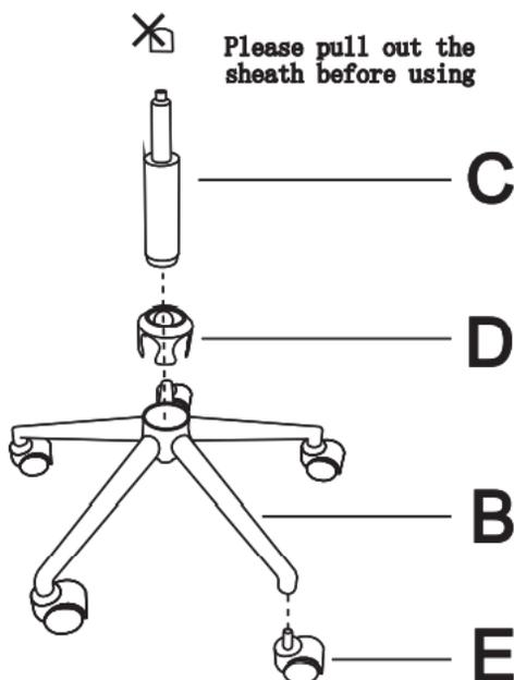
**STEP 3: Put the Part from step 1 on the Part from step 2**
